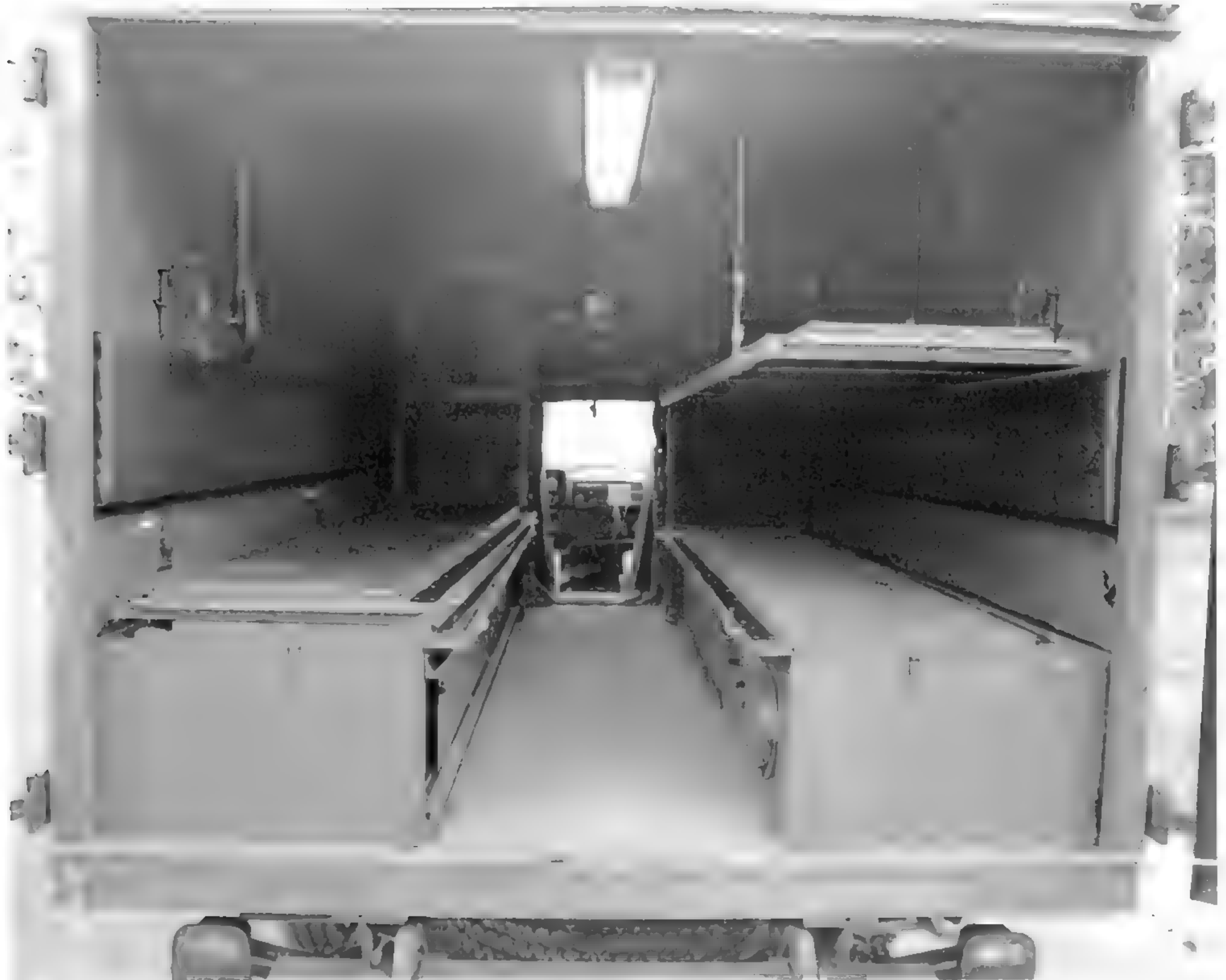
In this M1010, the right-hand side has been set up to transport two litter patients, and the left-hand side is configured to transport four ambulatory patients. (U.S. Army photo)
